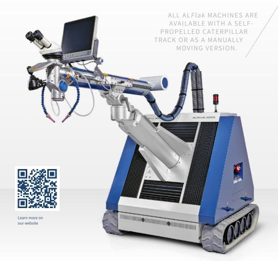
The **ALFlak** is also available with fiber laser sources: 300, 450, 600, 900 and even 1200 W. The fiber source model is recommended if your application requires a validated process, if you wish to weld using CW (continuous wave) method or pulses. For deep welding in sheet metal fabrication, for laser cladding. And also, for melting thick wire diameters up to 2.0 mm in the high performance classes.
