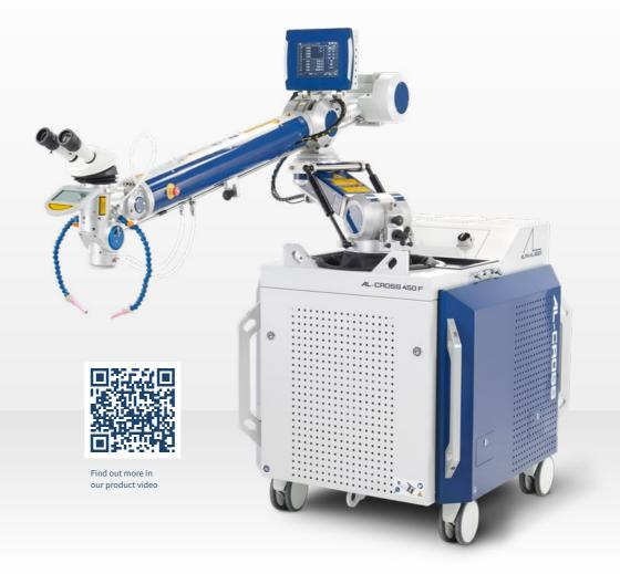
The AL-CROSS is ideal for use in sheet metal applications or in mechanical engineering. Equipped with a 600 W laser source, it is an entry-level system for "heavy metal" operations. Anyone who wants flexible pulsed or CW deep penetration welding - e.g. on large tanks gets the necessary laser power and flexibility with the AL-CROSS. The welding behavior can be influenced via predefined pulse shapes.
