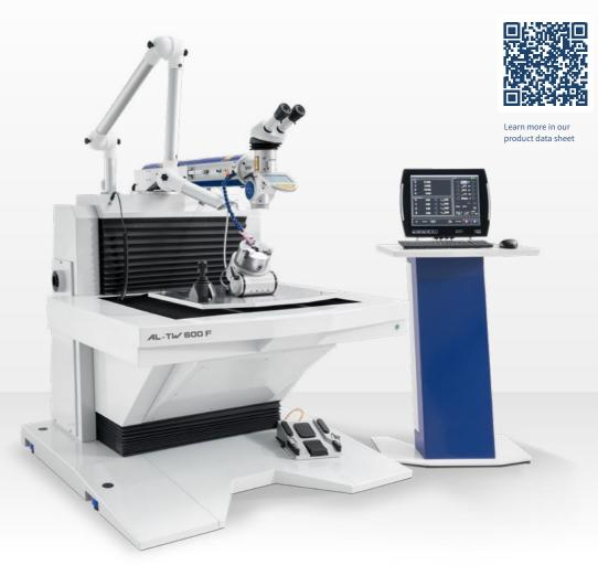
The **AL-TW** laser system has the laser source (Nd:YAG or fiber laser) integrated in the table. The workpieces can be precisely controlled in 3 axes (X, Y, Z) during welding. In addition, a rotary axis for circumferential welding is available as an option.
