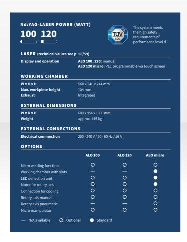
The **ALO** is the ideal device for anyone who wants to weld long or bulky parts quickly, manually and flexibly. It offers an easy loading and working in the shielded laser safety area.
